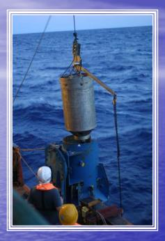
Driscoll Piston Corer 74mm diameter cores Up to 15m barrel length 1000kg bomb weight
