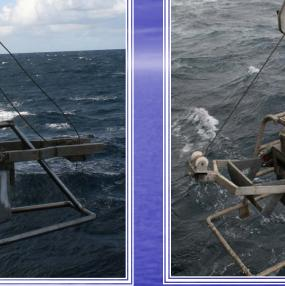
SMBA Box Corer 500x500mm square box 500mm box length 800kg weight
