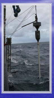
NIOZ Piston Corer 110mm or 90mm diameter cores Up to 21m barrel length 500, 1000 or 1500kg bomb weight
